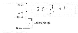
"DO NOT connect "DIM- to -V"
