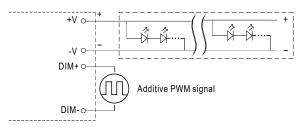
"DO NOT connect "DIM- to -V"
